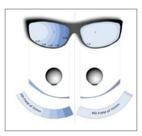
This image shows the difference between a conventional Single Vision Wrap lens and the Single Vision Wrap HD™ lens. In the conventional the pupil has an error of 0.25. However, Single Vision Wrap HD™ provides the wearer with accurate power in the pupil and in almost any gaze direction.
